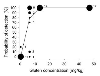
Figure 2. POD observed by each of 18 participating laboratories for samples extracted with Cocktail solution (part B) between 0.38 and 47.1 mg/kg gluten. Number stated at each circle means number of laboratories with the same POD. Areas of circles are proportional to number of laboratories.
